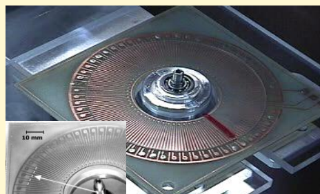
Electrostatic actuator for an atomic clock setup
